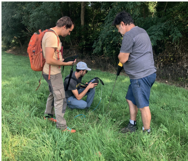
Figure 7 Soil gas measures with GA5000 in the North Pyrenean Frontal Thrust context (France) — H 2 NA project. Perforator is used in percussive mode to avoid artificial increase of H 2 content by drill bit rotation.
